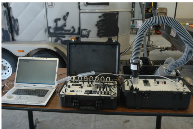
Figure 2: Field metabolic system (Sable Systems, Las Vegas, NV, USA) hooked up to a horse trailer and used for measuring rate of oxygen consumed and carbon dioxide produced for cattle confined to a horse trailer.
