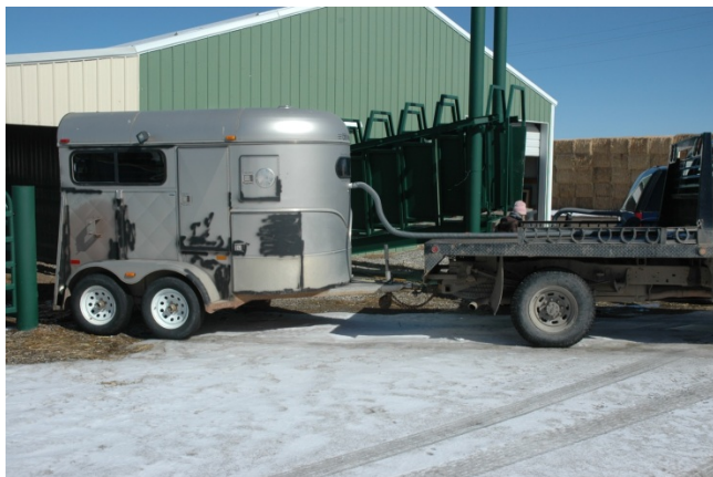
Figure 1: Horse trailer adapted as an indirect calorimetry system for measuring rate of oxygen consumed and carbon dioxide produced by cattle.
