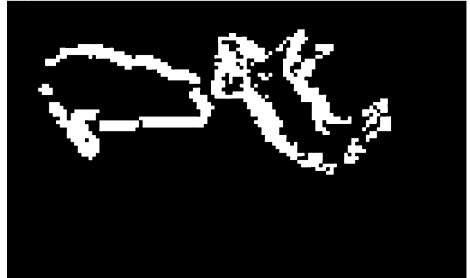
Figure 9. Result of the motion detection revealing movement of the top two pigs. Position of the third (bottom) pig remained unchanged.
