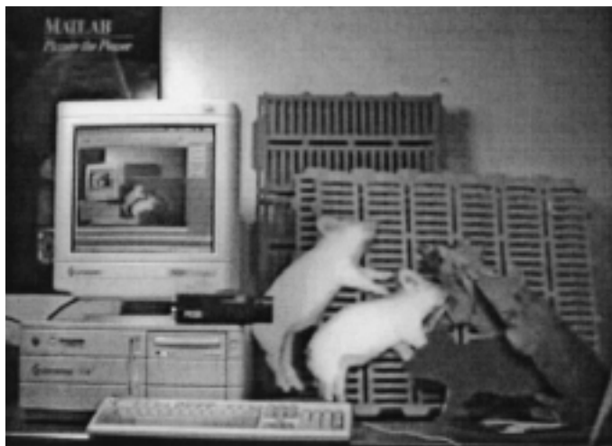
Figure 5. System components for development of automatic segmentation and selection of pig postural images, including a PC with an image grabber, a CCD video camera, commercial slat flooring, and artificial cartoon-cut pigs.
