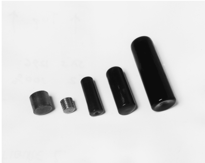
Figure 2. Various boluses developed for administering selenium to ruminants, from the left: the original iron/selenium pellet, steel “grinder” to eliminate organic coating, and soluble glass boluses for sheep and cattle.
